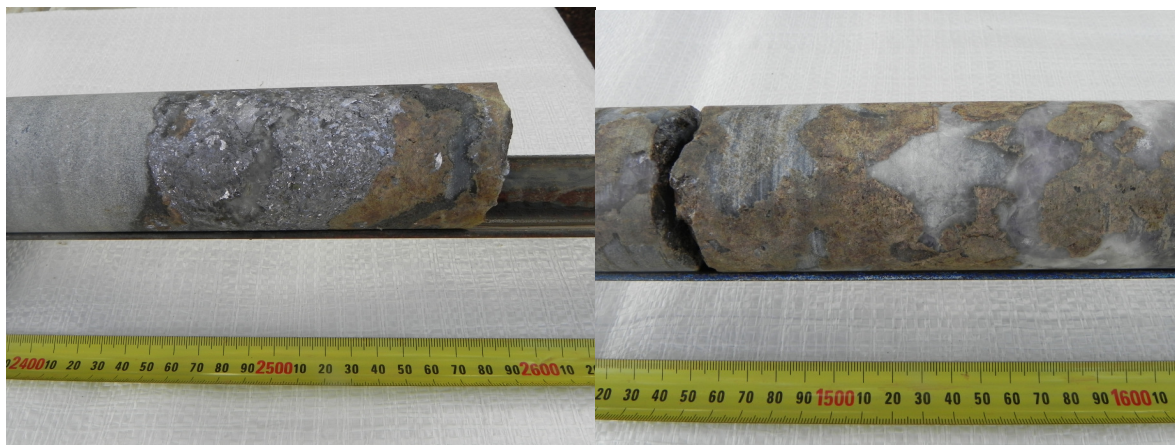
Figure 4. Photographs of high grade silver-rich galena (at 317.25m) and high grade sphalerite (at 316.25m) mineralisation from DF12.
